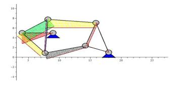
Figure 10 – The diagram of axial distributed inertial forces, originated from link weight of investigated mechanism
