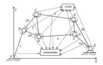
Figure 6 – Decomposing of structure into elements and joints
