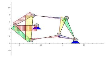
Figure 11 – The diagram of cross distributed inertial forces, originated from link weight of investigated mechanism
