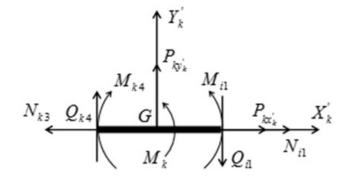
Figure 9 – Rigid joints of a link with a constant cross-sections of elements, where the external concentrated forces are applied
