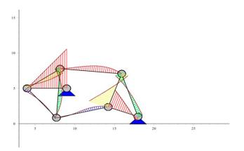
Figure 13 – The diagram of axial forces, originated from distributed inertial forces acting on links of mechanism with statically indeterminate structure
