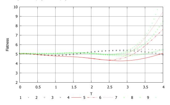
Figure 5: Comparison of the results of modeling the evolution of flatness, spectral and hybrid methods for modeling the Taylor-Green vortex of: TG short-time theory at: 1) Re=100; 2)Re=300; 3)Re=600; Spectral method,  $256^3$  at: 4)Re=100; 5)Re=300; 6)Re=600; HFD method at: 7)Re=100; 8)Re=300; 9)Re=600.
