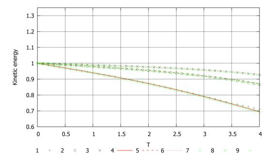
Figure 2: Comparative results of modeling the evolution of the average kinetic energy in time, spectral and hybrid methods of modeling the Taylor-Green vortex of: TG short-time theory at: 1) Re=100; 2)Re=300; 3)Re=600; Spectral method,  $256^3$  at: 4)Re=100; 5)Re=300; 6)Re=600; HFD method at: 7)Re=100; 8)Re=300; 9)Re=600.
