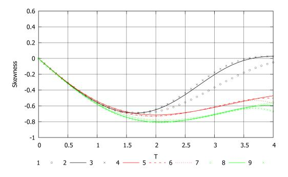
Figure 4: Comparison of the results of modeling the evolution of skewness, spectral and hybrid methods for modeling the Taylor-Green vortex of: TG short-time theory at: 1) Re=100; 2)Re=300; 3)Re=600; Spectral method,  $256^3$  at: 4)Re=100; 5)Re=300; 6)Re=600; HFD method at: 7)Re=100; 8)Re=300; 9)Re=600.
