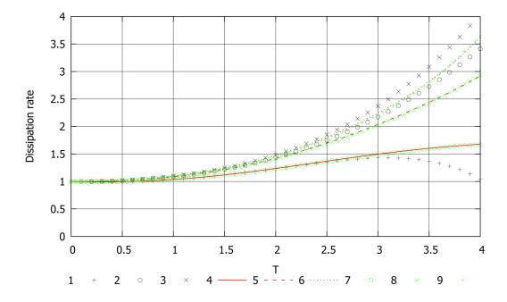
Figure 3: Comparative results of modeling the evolution of the average rate of dissipation of the decay of turbulence in time, the spectral and hybrid methods of modeling the Taylor-Green vortexof: TG short-time theory at: 1) Re=100; 2)Re=300; 3)Re=600; Spectral method,  $256^3$  at: 4)Re=100; 5)Re=300; 6)Re=600; HFD method at: 7)Re=100; 8)Re=300; 9)Re=600.
