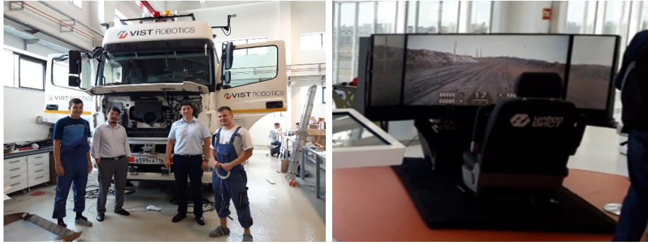
Figure 1: Autonomous truck based on KAMAZ Neo 5490 platform (left) and Remote control cabin designed by VIST Group (right)
