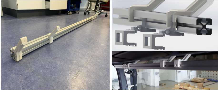
Figure 2: Finished assembly of fasteners for the cameras
