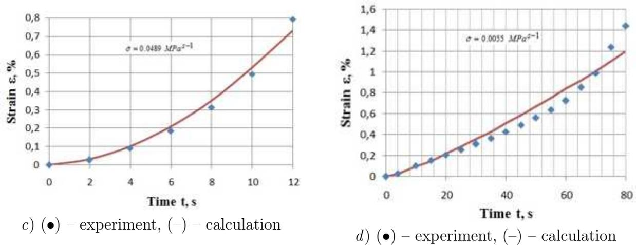
Figure 7: Graphs of strain variation in time at various loading rates
