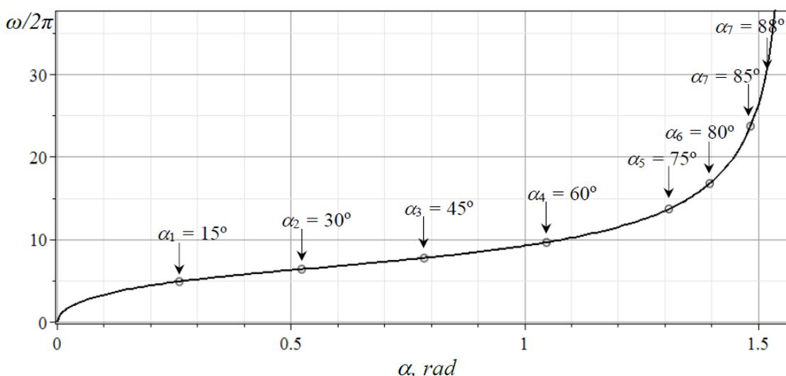
**Figure 3** - Dependence between the angular velocity and the angle of inclination
