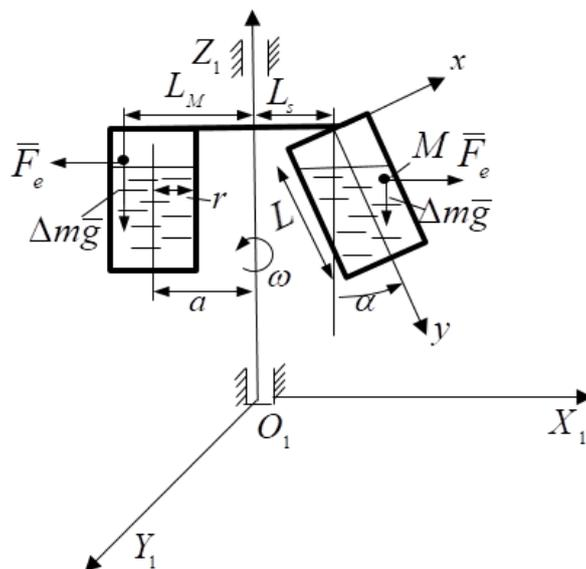
**Figure 2** - Scheme of the rotor system
