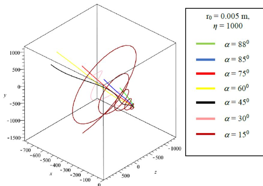
**Figure 4** - Movement of the particle at different values of the slope of the tube
