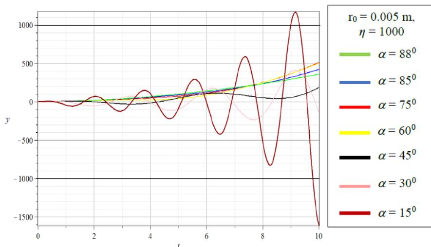
**Figure 5** - Movement of a particle at different values of the inclination of the tube along the longitudinal axis as a function of time
