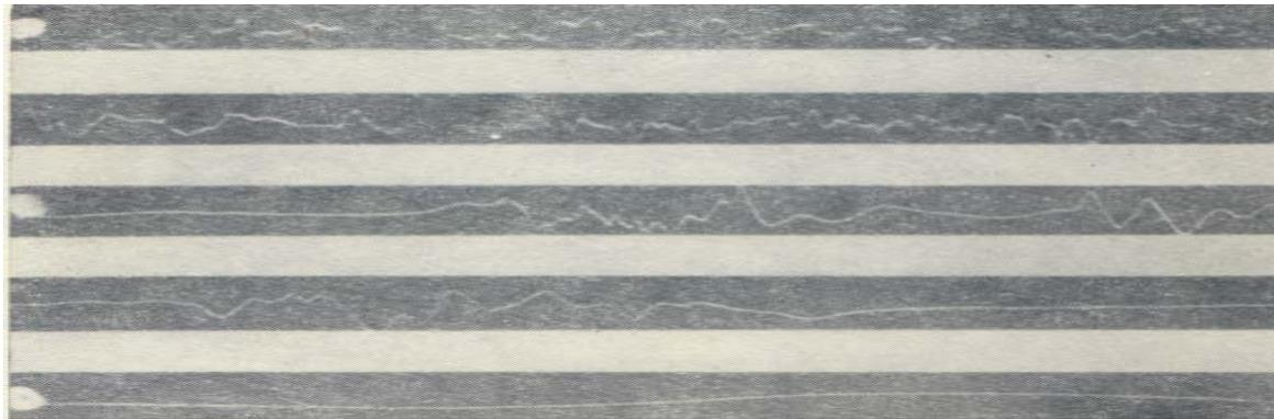
Рис. 4: Oscillograms of momentary velocity's value at the various points of turbulent jet, [19]. During the movement of the sensor from the center of jet to periphery developed turbulent flow (two pictures from above) is replaced by the intermittent (two average pictures) and potential (below) flow.
