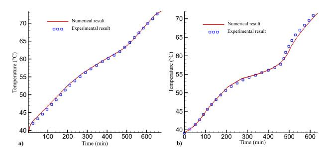
**Figure 8** – Comparison of the experimental and numerical results for charging LHT with PCM. Oulet temperature (a) and temperature at middle position in PCM container (b)
