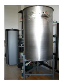
Figure 2 – Latent heat storage which contains 39 PCM containers filled with E53
