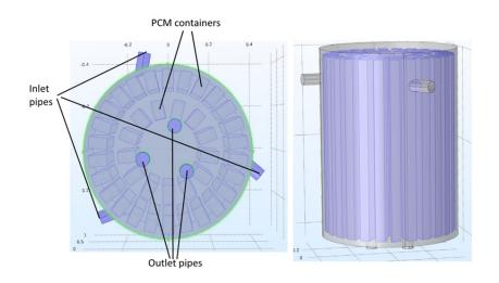
Figure 4 – Design features of the latent heat storage
