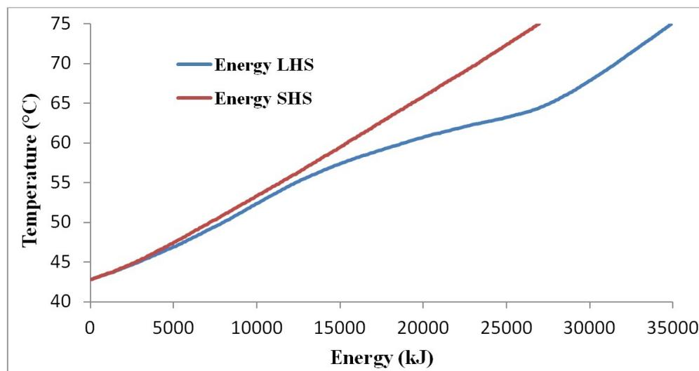
**Figure 9** – Temperature histories of HTF during SHS and LHS charging process
