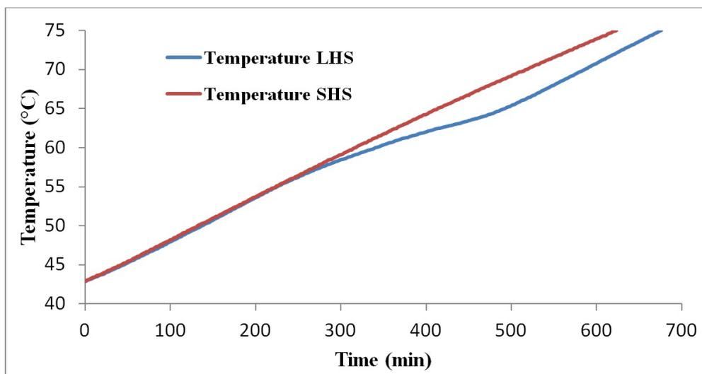
**Figure 6** – Temperature histories of HTF during SHS and LHS charging process
