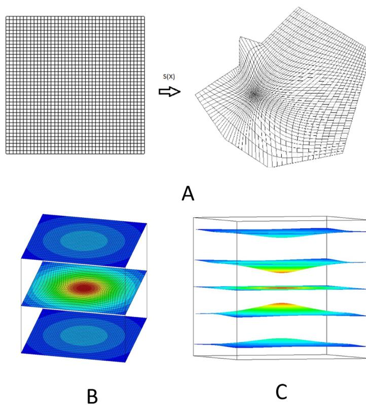
**Figure 2** - Structured grid construction: A) mapping demonstration; B-C) using reversed Beltrami equation, control function is presented by colors
