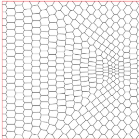
**Figure 4** - Example of unstructured grid constructed using adaptive close regular points set
