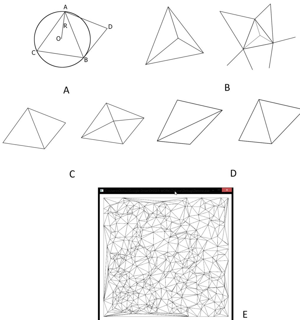
**Figure 1** - Delaunay triangulation: A) Delaunay principle; B) Delaunay construction: adding new point in triangular cell; C) Delaunay construction: adding new point to existing edge; D) flip operation; E) demonstration of constructed triangulation on the random 100 points
