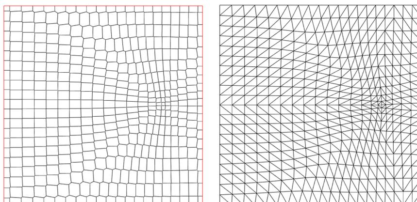
**Figure 3** - Example of unstructured grid constructed using points set defined by nodes of adaptive structured grid: left – Voronoy diagram and right – Delaunay triangulation
