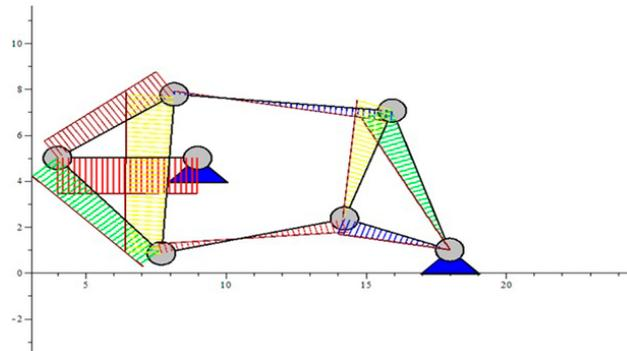
**Figure 11** – The diagram of cross distributed inertial forces, originated from link weight of investigated mechanism
