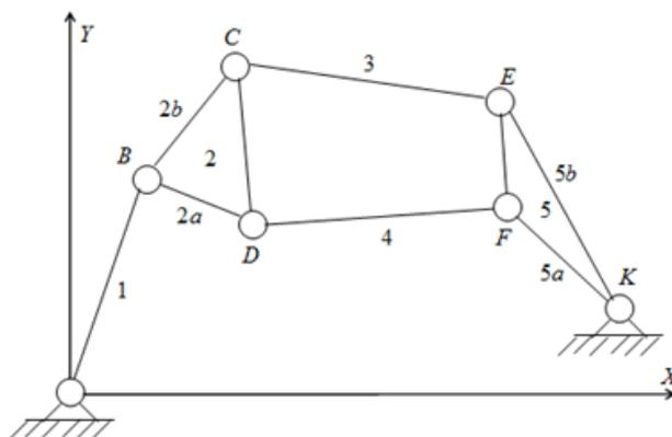
Figure 4 – The fourth class planar mechanism
