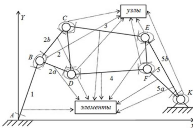
Figure 6 – Decomposing of structure into elements and joints
