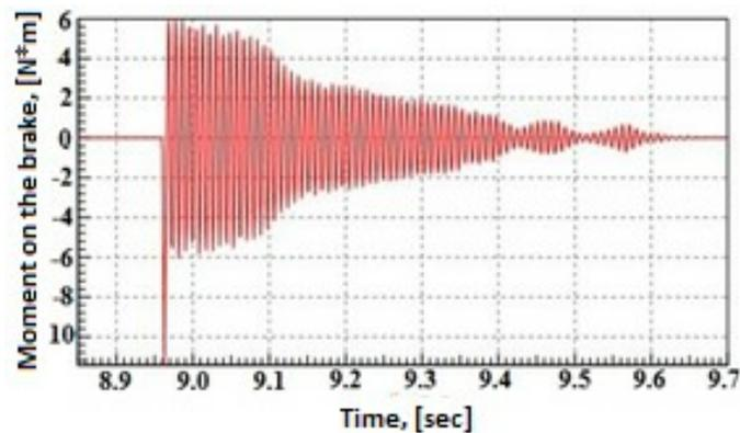
Figure 10: Moment on the brake when switching-on
