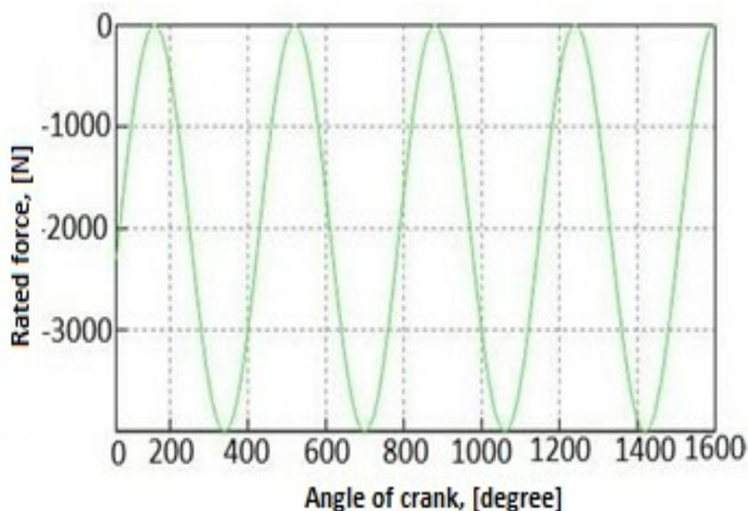
Figure 4: Rated force, developing by the slider of the slider-crank working mechanism
