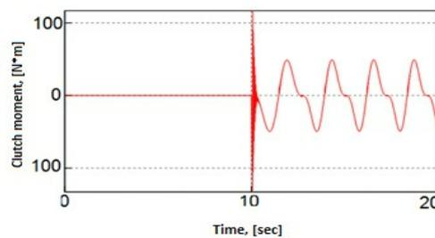
Figure 6: The moment transmitted by the start clutch
