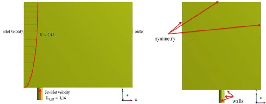
Figure 3: Basic conditions for the vertical view of the reactor in the OXY plane; Basic conditions of the vertical view of the reactor in the plane of OYZ
