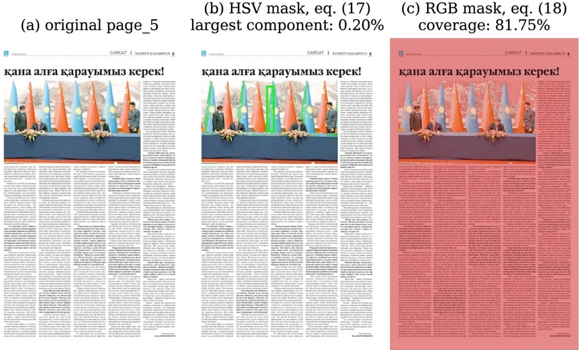
Figure 5: Colour-aware segmentation on a representative newspaper page. (a) Original page. (b) HSV mask with (dH, dS, dV) = (8, 60, 60) . (c) RGB mask with \tau_{\text{RGB}} = 30 .
